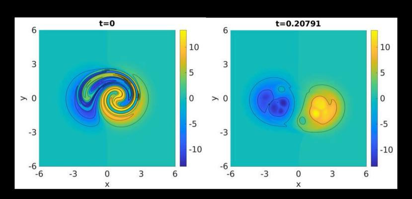
We see this 2D model is able to capture the main topological feature of the original 3D simulation. The initially highly braided pattern (left) is able to relax to a simple state (right), which corresponds to the two oppositely twisted flux tubes.
